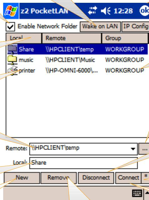
Click here to show [IP Config Dialog](#). You can check IP Configuration, release/renew IP, ping and change IP settings with IP Config Dialog.
